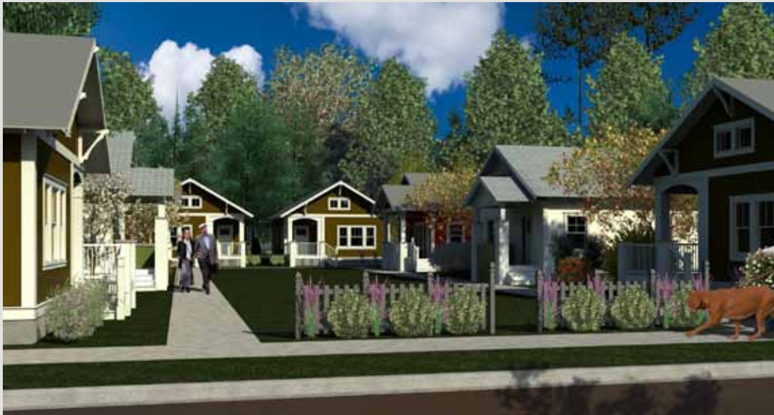
This image illustrates a hypothetical cottage court located within Red Bud Village. Cottage courts, sometimes referred to as bungalow courts, include relatively small cottages that are grouped to face towards a common pedestrian green space, with parking and services occurring behind. This helps to reduce the size of individual private yards while still providing an attractive amenity for the residents. Because of their arrangement, cottage courts can achieve significant densities (10-20 units to the acre) and yet compliment and coexist with other less intensive land uses. This helps to make more use of local infrastructure while preserving a certain quality of life. Cottage courts are popular with seniors, students, empty nesters, singles, and young families because they decrease private maintenance and are more affordable. They can also be adapted for agricultural workers.
