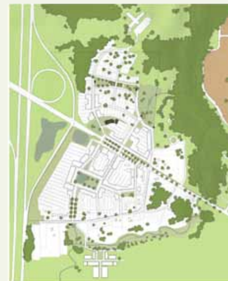
This diagram illustrates the location of open space and public space. The network of streets, parks, squares, and plazas has been designed to help drain the site more naturally, which limits stormwater pollution and inlet-and-pipe infrastructure.
