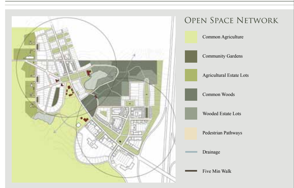
The diagram above illustrates the plan's open space network, preserves, and agricultural and woodland estate lots. Also visible is the reinforced natural drainage pattern, which uses two ponds to help control stormwater and double as attractive amenities.
